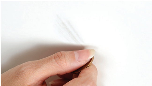
Photograph 1: Appearance of the white scratch-like stain left by a fingernail
