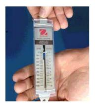
Figure 5. Zeroing the Scale
