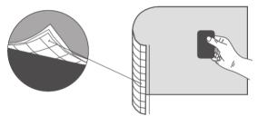
Figure 1: 3M™ Comply™ Air-Release Channels
